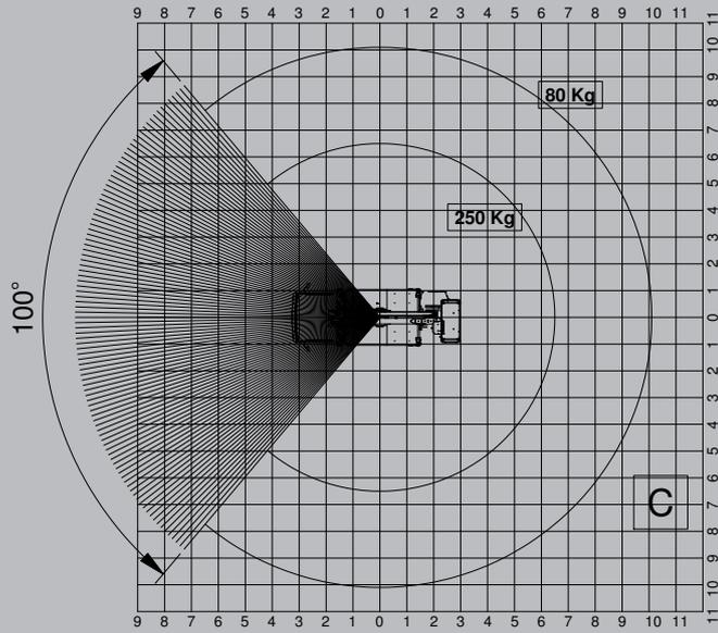
**CROSSBEAMS ONE SIDE FULLY OPENED ONE SIDE CLOSED**
